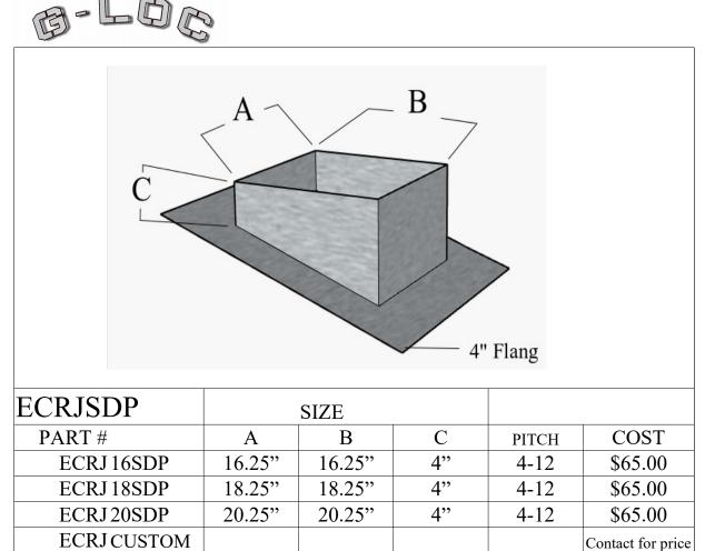
Description: Pitched AC flashing (no damper) used with G-LOC ECEL, and ECDUCT---S Construction: 26ga G90 galvanized spot welded seams.
