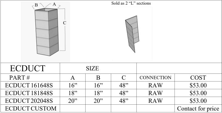
Description: Straight rectangular duct, with out liner. For use with G-LOC AC flashing
